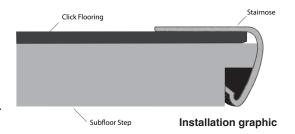
**Step Three:** Using an adhesive appropriate for bonding two non-porous surfaces together, glue the stair nose to the edge of the installed flooring.
